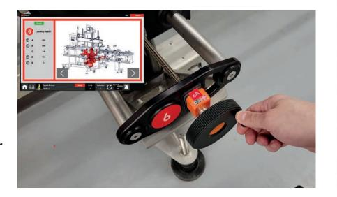
in the screen to the corresponding color and letter on your machine. And when done, that recipe is saved in the HMI and ready to be recalled at the push of a button for a ridiculously quick and easy replication.
