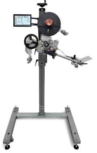
The NITA 100% servo driven stand-alone labeling head is made for applying labels to whatever, whenever. Geek out on up to 3200 inches per minute of super accurate label application.
