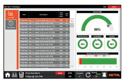
Every NITA includes a live S.C.A.D.A. dashboard allowing for real time O.E.E. data and other production efficiencies like uptime, downtime, changeover times and container and label usage to be viewed right from the comfort of your Panel PC HMI or via OPC/UA connectivity.
