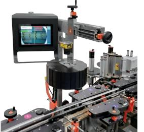
Professional grade cameras or sensors married to servo motor-driven belt systems rotate both round or square containers. Available integrated into a powerful NITA Labeler or as a convenient Stand-Alone Orientation System when a label application is not needed.
